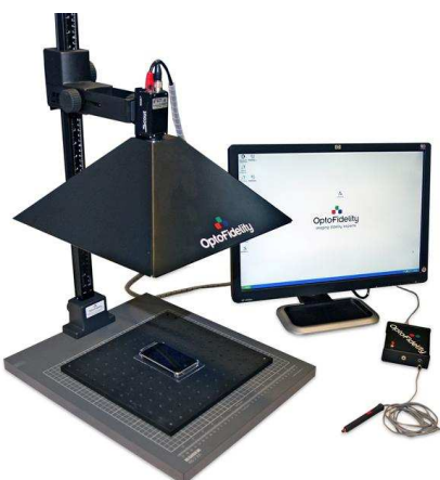
Test set up to measure operations from user interface.
